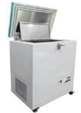
Cooling Chamber for Impact test.
